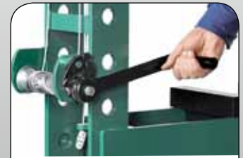
Fast and safe adjustment of the press table height, using a braked winch.
