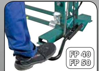
Foot operated for hands-free operation under load.
